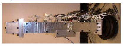
Acoustic liners are used to reduce the noise radiated from aircraft engine nacelles. They are also applied in augmentors ducts to absorb acoustic energy to prevent combustion instabilities. The liner
