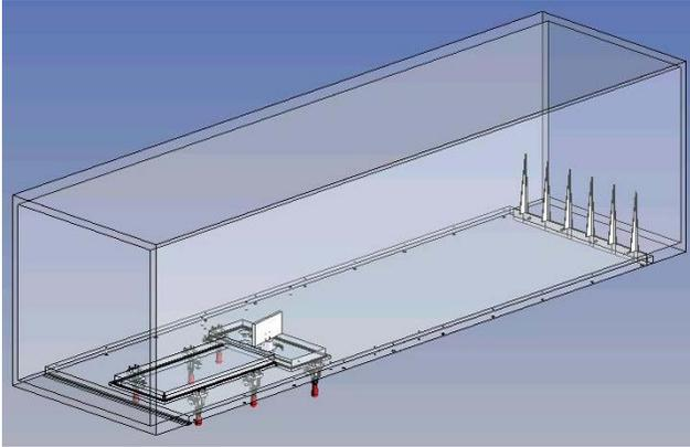
Experiments are performed in a subsonic wind tunnel with a special test section that is used to study unsteady flow separation behind generic protrusions to simulate flight conditions of an airplane with appendages installed on the fuselage (cameras, antennas, probes, etc). The experiments enable research of the correlation between the flow field, unsteady pressure, and vibrational modes induced on a fuselage panel.
