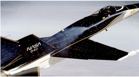
Lift force on delta wings at a high angle of attack relies on large-scale vortices that separate at the leading edges of the wing. At high angle of attack these vortices lose gradually their coherence due to intrinsic flow instabilities that lead to vortex breakdown. At these conditions, the lift produced by the vortices is reduced causing loss of controllability and stall.
