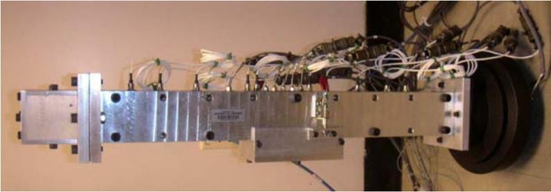
Acoustic liners are used to reduce the noise radiated from aircraft engine nacelles. They are also applied in augmentors ducts to absorb acoustic energy to prevent combustion instabilities. The liner
