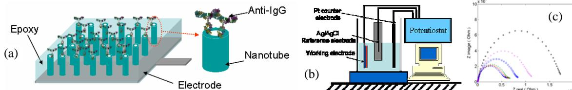
Figure 1. Electronic Biosensor: (a) structure of the immunosensor; (b) EIS experimental setup; and (c) example electrochemical impedance spectra for different concentrations of antigen on nanotubes.
